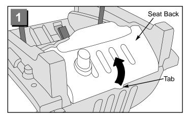
Lift the tab on the back of the seat back to unlatch the peg from the hole in the vehicle body.
